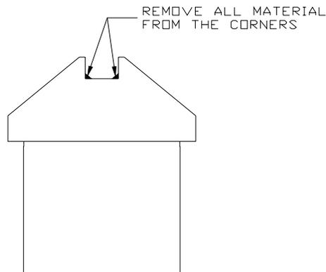
point loading. This can be done on a grinder with a green wheel installed. (Green wheel stones are used to grind carbide.) Cee-Jay Tool, LLC sends out carbide pre-ground.
